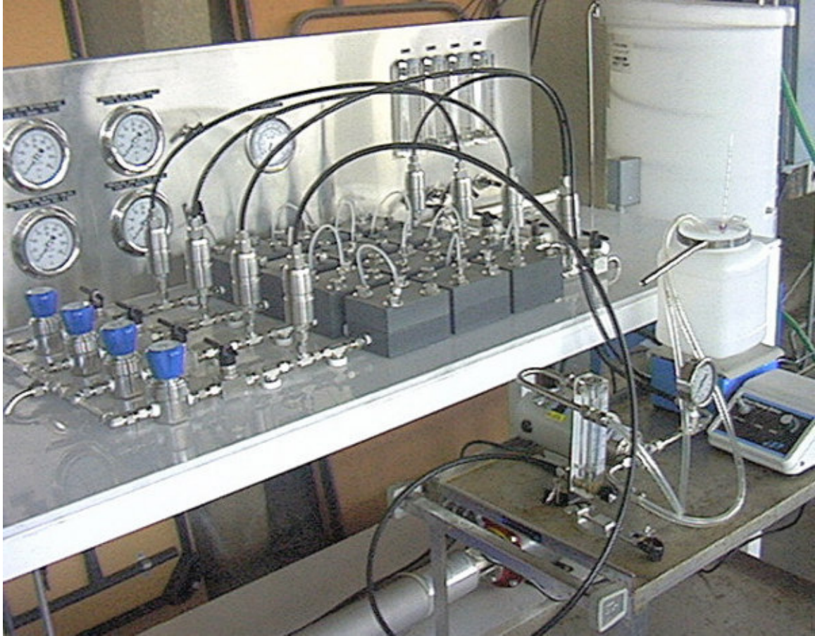
Figure 3. RO cleaning cycle bypass with cleaning agent recirculated over the surface of the membranes. Note detergent heating coil is missing from this picture.
